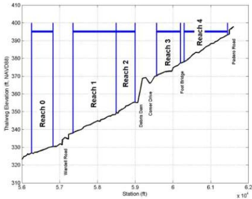
**Figure 2.A-7. Definition of reaches 0- 4 relative to the thalweg profile for the existing conditions. Thalweg elevation data were obtained from the 2006 HEC-RAS model**
