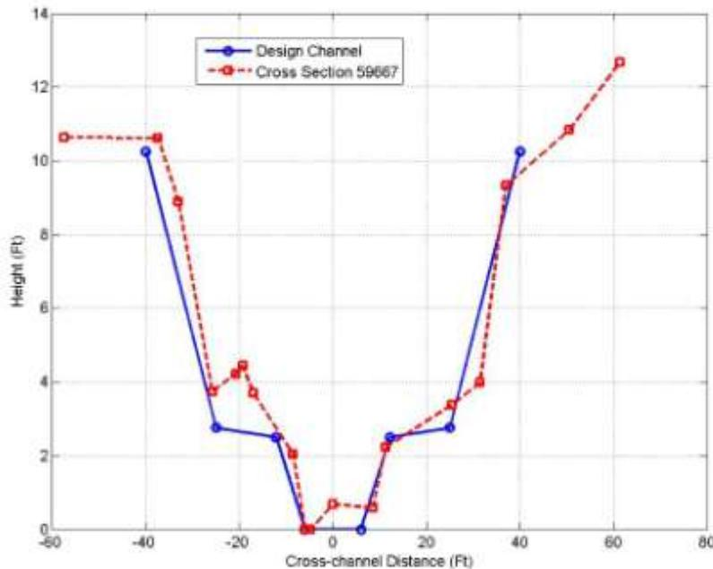
**Figure 2.A-8. A channel cross section located about 500 feet upstream of Comer Dam superimposed on the design channel**
