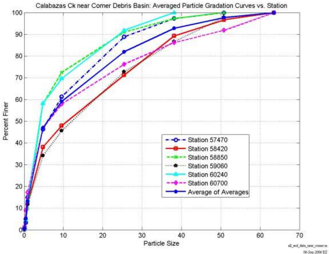
**Figure 2.A-3. Averaged sediment profiles at 6 stations near Comer Debris Dam. The “average of averages” (i.e., the average of the 17 samples collected near the project site) profile was used in calculations of sediment transport capacity for each reach of channel**
