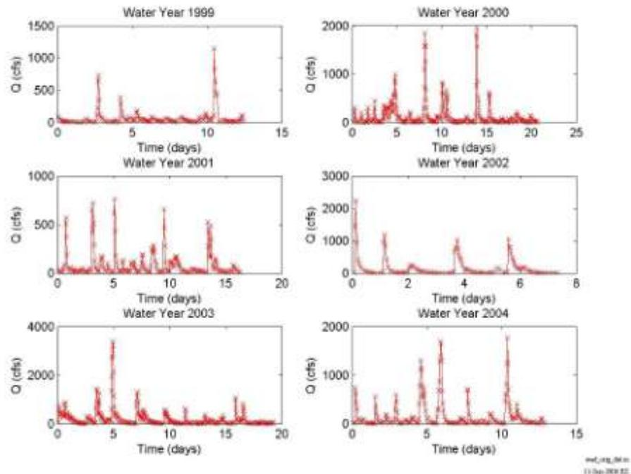
**Figure 2.A-1. Flow Data at Wilcox Gauge Station for water years 1999 – 2004. Zero flows have been removed from the record, which is treated as a continuous flow record for the purposes of our sediment transport analysis.**
