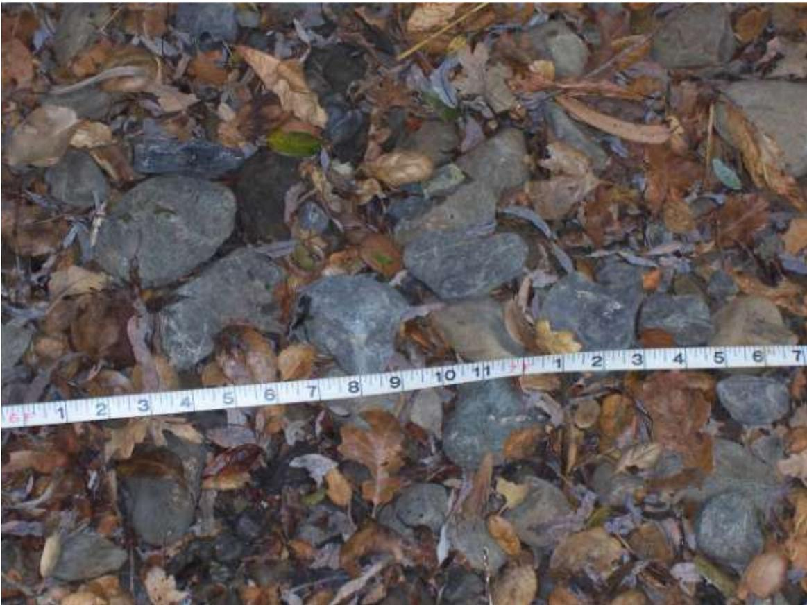
**Figure 2.A-6. Bed sediments in a riffle in Reach 2. Bed appears to have about 80 percent covered by armor (in the riffles) Station 58670**
