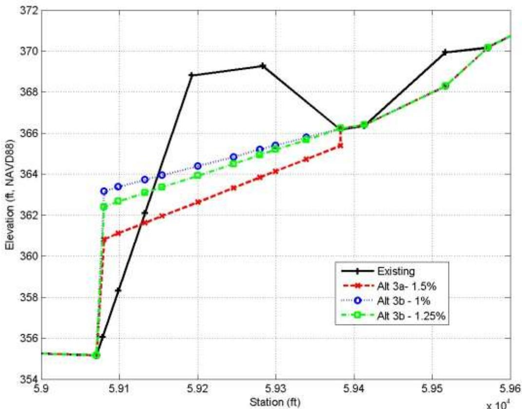
**Figure 2.A-9. Bed profiles developed for Alternative 3. The profiles for Alternatives 3a, 3b and 3b1 show the profiles used in each successive iteration of the equilibrium slope procedure**
