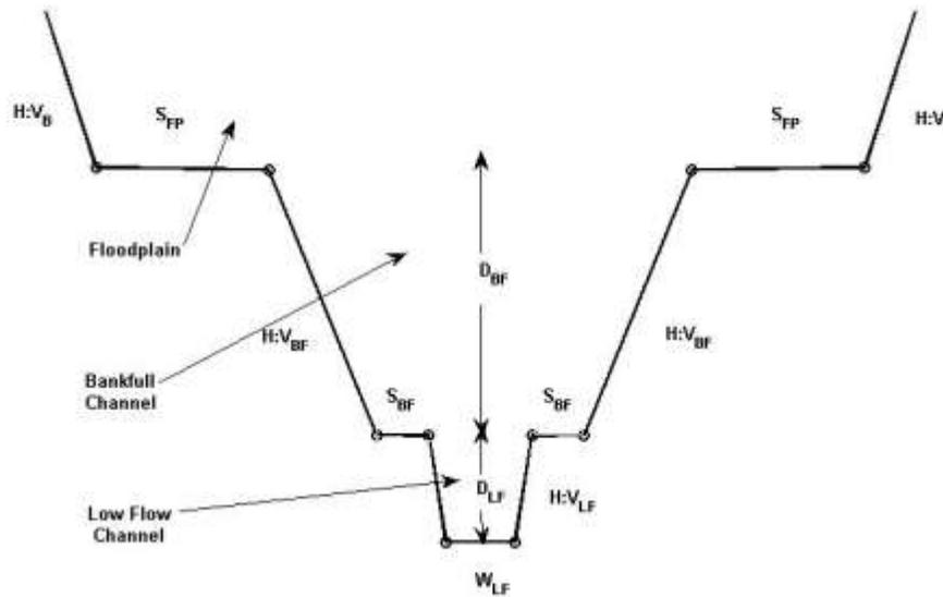
**Figure 2-1. Definition Sketch of a Compound Trapezoidal Cross-Section**
