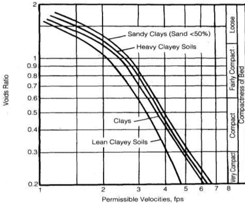
Figure 2-3a. Permissible Velocities for Cohesive Materials [ASCE 1992]
