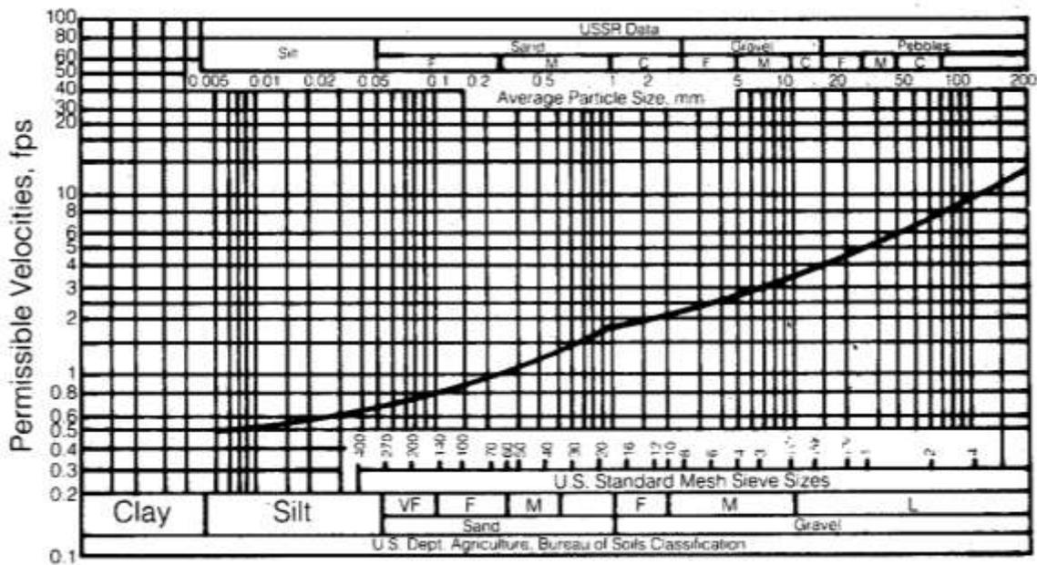
Figure 2-3b. Permissible Velocities for Non-Cohesive Materials [ASCE 1992]
