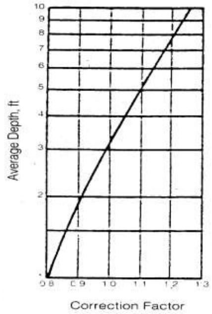
**Figure 2-3c. Correction Factor for Depth Effect**
